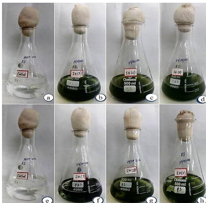
Plate 9.2. Biological treatment (6 weeks) of LDPE polythene films (a-control, b, c, d- Phormidium lucidum , e-control, f, g, h- Oscillatoria subbrevis )
