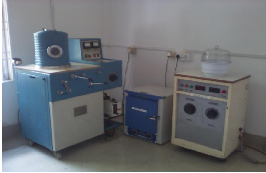
Figure 2.5 (a): Vacuum coating set up of OLED fabrication
