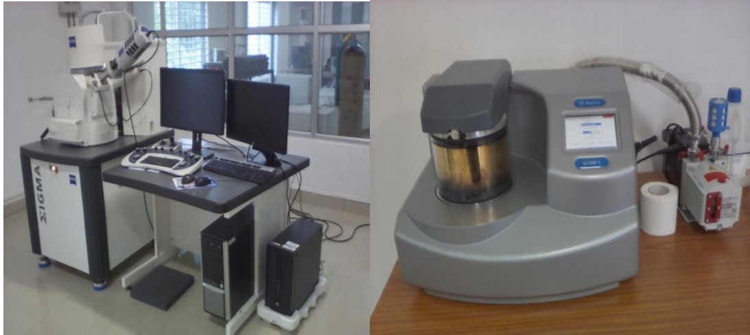
Figure 2.7 (b): Field emission SEM setup Figure 2.7(c): Gold coating unit under vacuum
